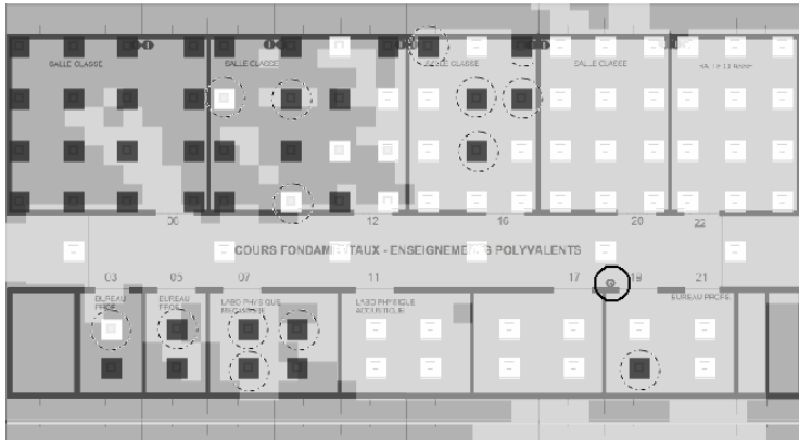
Fig. 16. Superposition of the measured and predicted “Interactive service” coverage maps. The white squares represent the location with sufficient coverage. The dark squares represent the location with insufficient coverage. The 11 dotted circles show the locations where prediction errors occurred (out of 94 measurement points).
