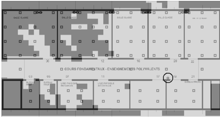
Fig. 15. Predicted “Interactive service” coverage in light grey. The access point is at the center of the black circle. The PixelFlow parameters are as in Fig. 13.
